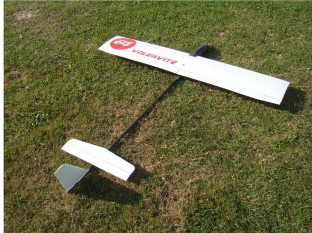
*A small racer (1m span, 300w only) where the fuselage length is longer than the span. Despite the fact that this configuration disturbs our minds, it is not so unusual for real racer planes. The fuselage increase allows to reduce fin and tail dimension (and then drag) and to increase the stabilities. Flight is like an arrow (on a rail).*
