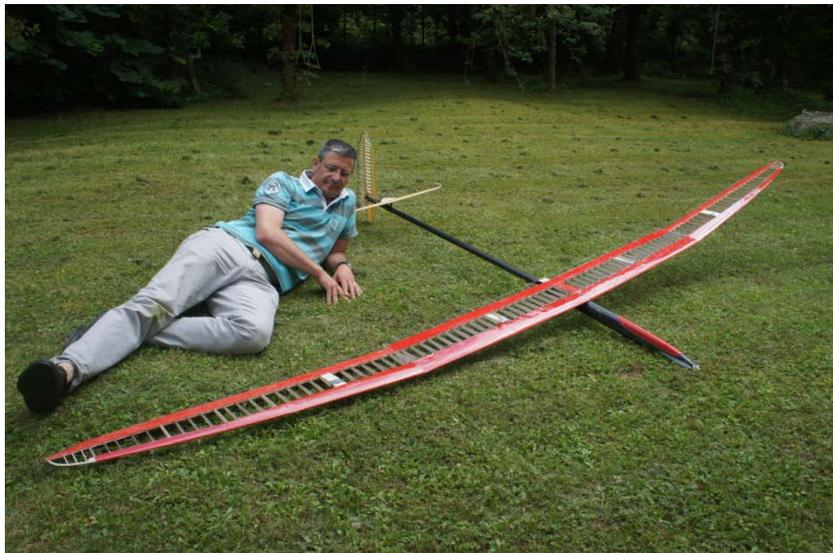
***The man is 1.93m long. Quiet a plane no? The Genoma<sup>2</sup> ends at 1.6/1.7kg. It is 300g lighter than the Genoma for greater span and surface... The Genoma<sup>2</sup> is also be able to make the barrels in circles or any other aerobatic maneuver.***
