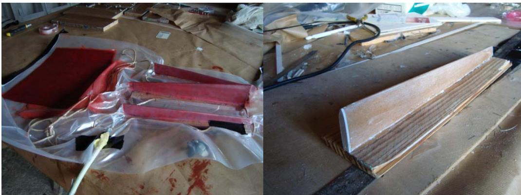
**How to mould the D-boxes ? Easy. On a positive mould. No much sciences behind. For wing 2 layers Kevlar of 60g/dm<sup>2</sup> is fare sufficient (the wing can support all aerobatics manoeuvrals). For tails and fin, a 60g/dm<sup>2</sup> kevlar is right OK.**
