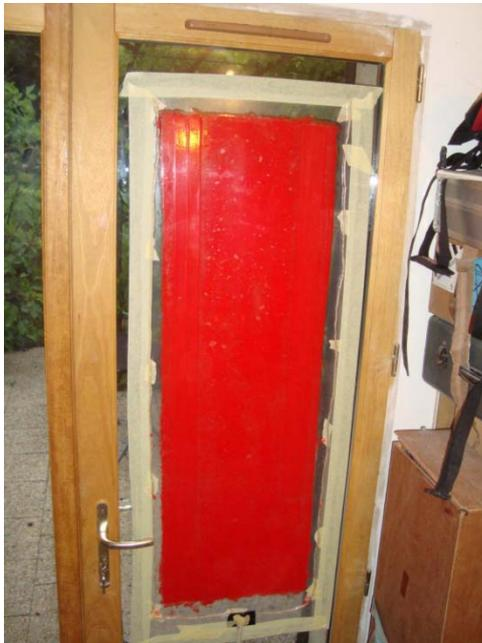
***How to mould the Flaps and ailerons D-Box: On a window! Do not forget to "wax" it.***
