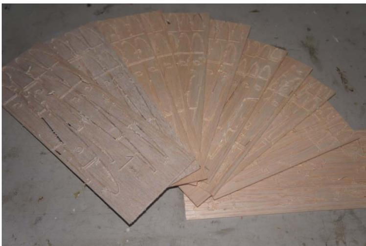
All Balsa wood pieces have been realized on a CNC machine. Of course, on request, files can be provided.
