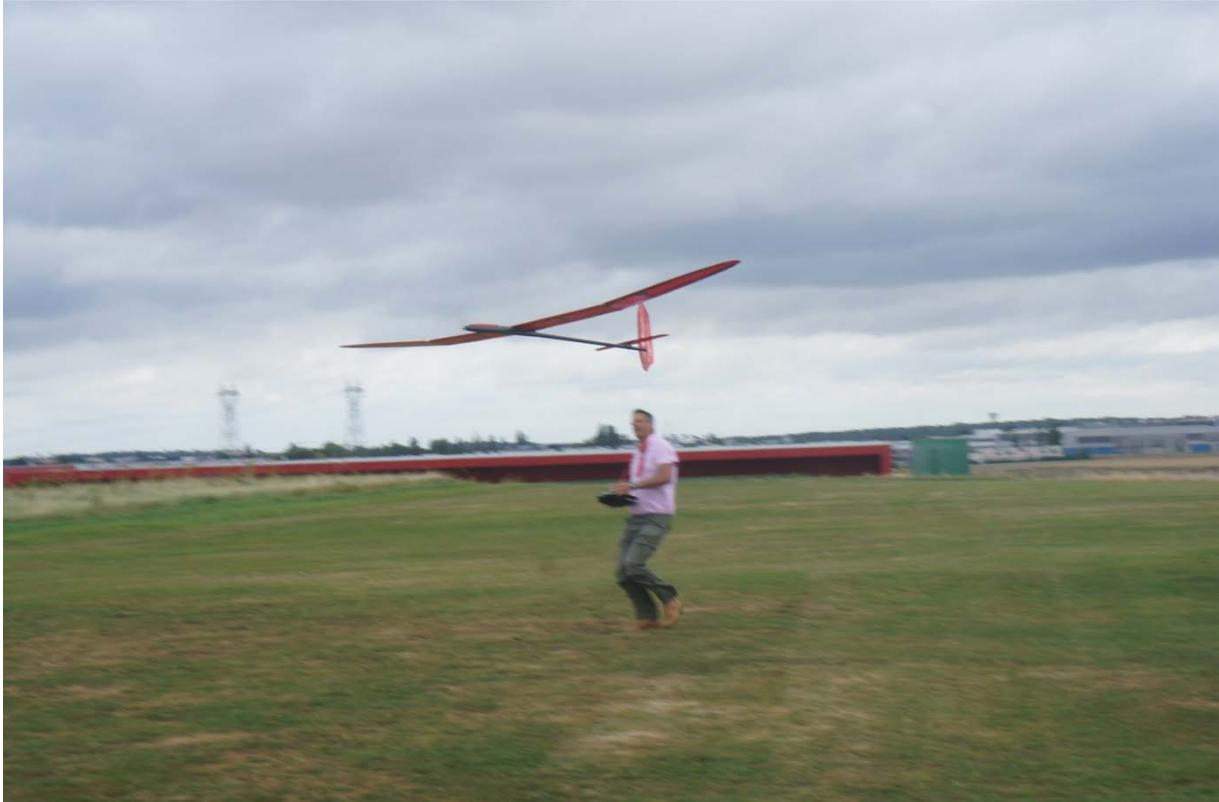
*Genoma<sup>2</sup> for its first flight. Except few adjustments, it flies perfectly and I found immediately comfortable. It is even better in circling ability due to the possible low wing load (19g/dm<sup>2</sup> without ballast). Of course things needs adjustment (compensation, trim...).*
