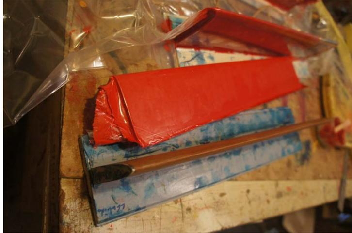
*View of D-box mold under process. On top, you can see the D-box bagged, in the center the D-box results and in the bottom of the picture the D-dox mold.*
